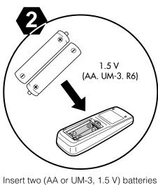
Insert two (AA or UM-3, 1.5 V) batteries into the remote control. Position the positive and negative ends of the batteries as indicated.
